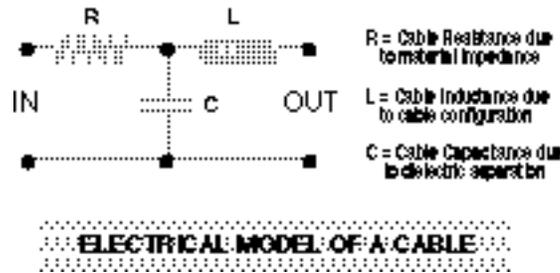
impedance (resistance to current flow.) For example, the impedance of RG-6 coax cable is supposed to be exactly 75 Ohms. The manufacturers of Audio/Video equipment design their units to match the impedance of the cables connected.
